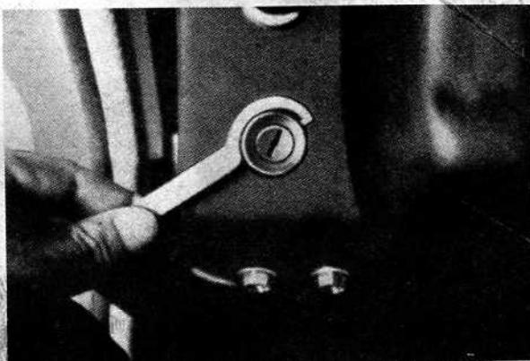
Removing the ignition switch trim ring with a spanner wrench
